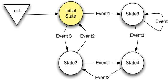
Fig. 3: A simple state space with four states
