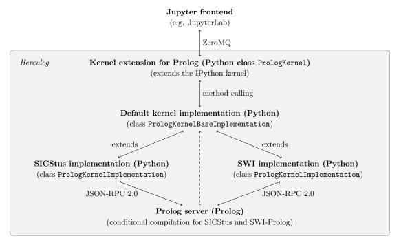
Figure 23: Diagram showing the architectural components and their communication methods.
