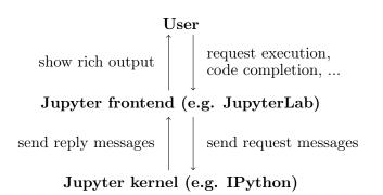
Figure 2: Diagram showing the handling of user interaction with a Jupyter frontend.
